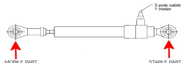
Attach the potentiometer through the ball joints positioned at the extremities, the sensor will measure the movement of the parts to which the ball joints are attached.
